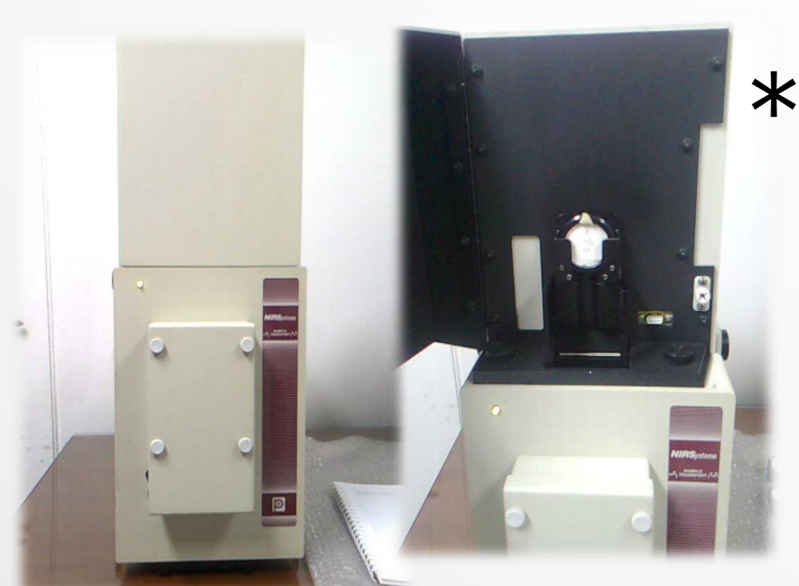
Fig. 2 FOSS-NIRSystem II monochromator model 6500, spectral range 400 to 2500 nm, in reflectance. * To the right: inside view
