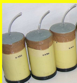
Figure 3: Lab scale silos (PVC tubes)
