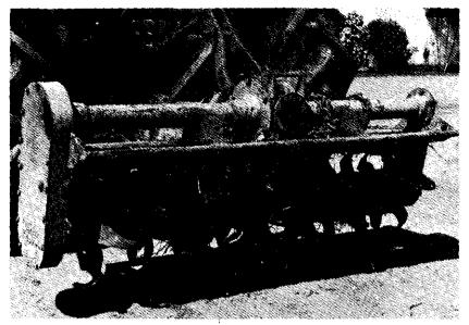
Photo 2: Rototiller designed for both wet and dry fields.
