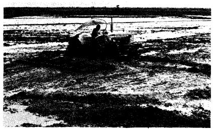
Photo 12: Leveling and finishing of field with the spike tooth harrow
