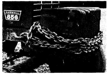
Photo 1: Front weights, chain and pull points to stabilize the tractor and for pulling when stuck in the mud.
