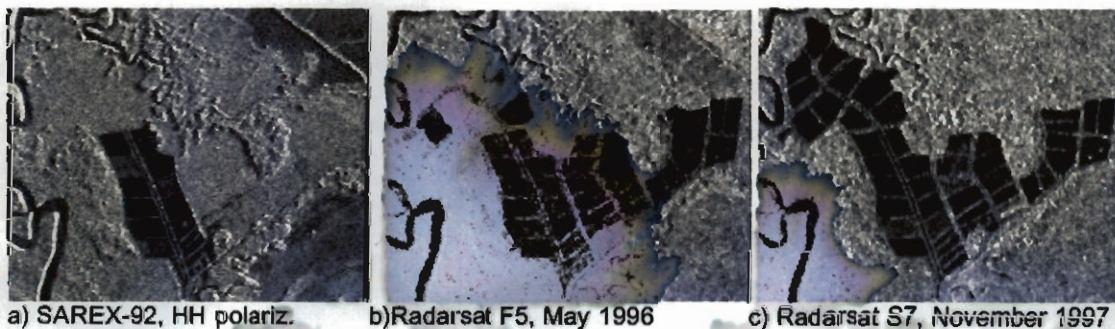
Figure 1: 3.85 km wide portion of the Térraba-Sierpe test site illustrating the expansion of shrimp ponds
