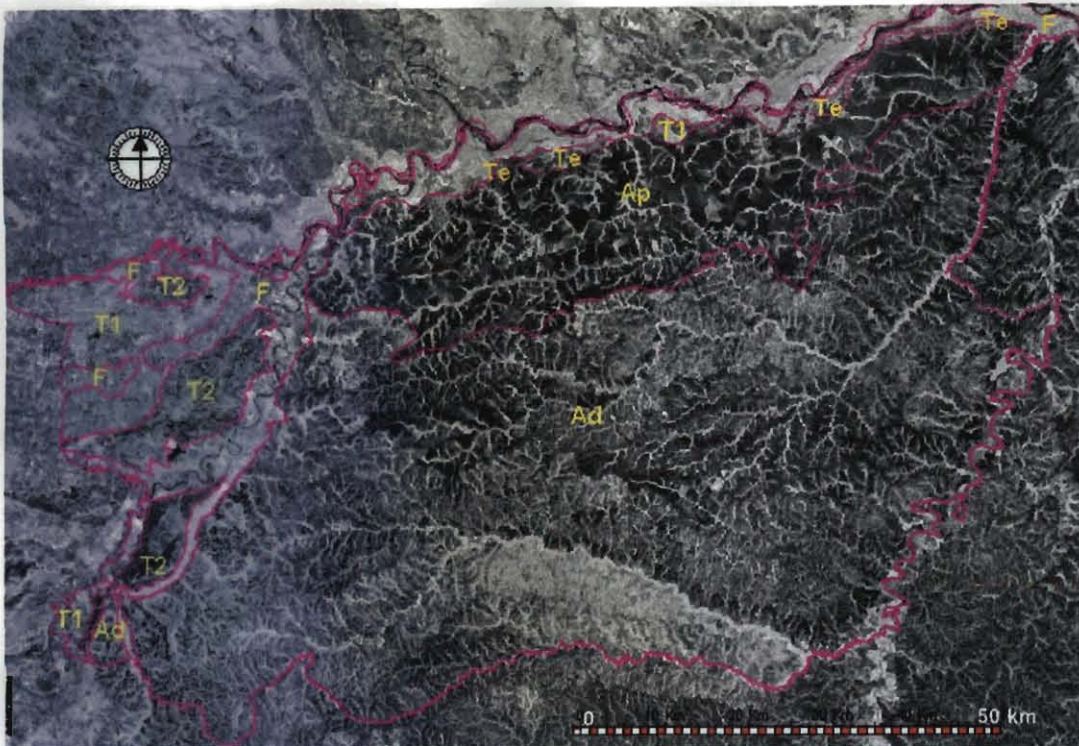
Figure 3: General map of landscape types overlaid on a portion of a mosaic of JERS-1 images acquired in 1995 (©NASDA, 1998), over the municipality of Puerto López. Landscape types presented are the flat high planes (Ap), the dissected high plains (Ad), depositional alluvial terrasses (T1 and T2), floodplains (F) and erosional terrasses (Te).
