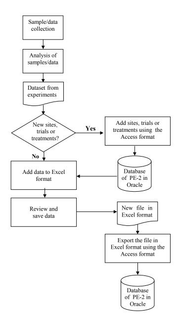
Figure 35. The process of compilation and storage of data for each sample/ observation from Soils project (PE-2).
