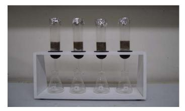
Picture 12. Leaching Tube Setup.
