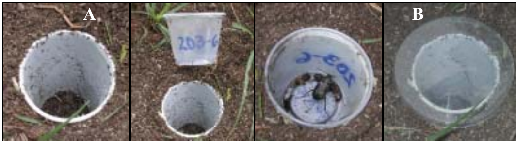
Figure 1.18.1.2. (A) Fixed component and removable component and (B) lid of the pitfall traps in the field.
