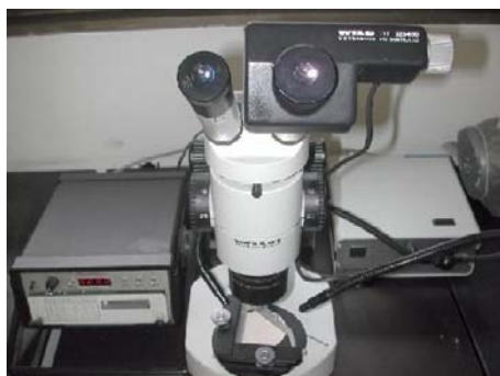
Figure 5. Digital micrometric measuring devise to determine morphological size of Aleurotrachelus socialis immatures.
