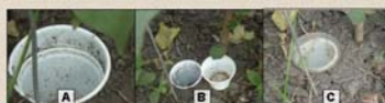
Fig. 1. Pitfall traps showing (A) fixed component, (B) removable component and (C) lid.
