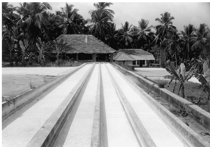
Fig. 15.1. Settling of starch in a small factory.
