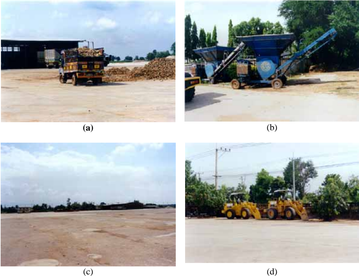
Figure 7. Chips processing : (a) Root transportation (b) Conveyor and chopper (c) Drying area and (d) Turning chips by tractor
