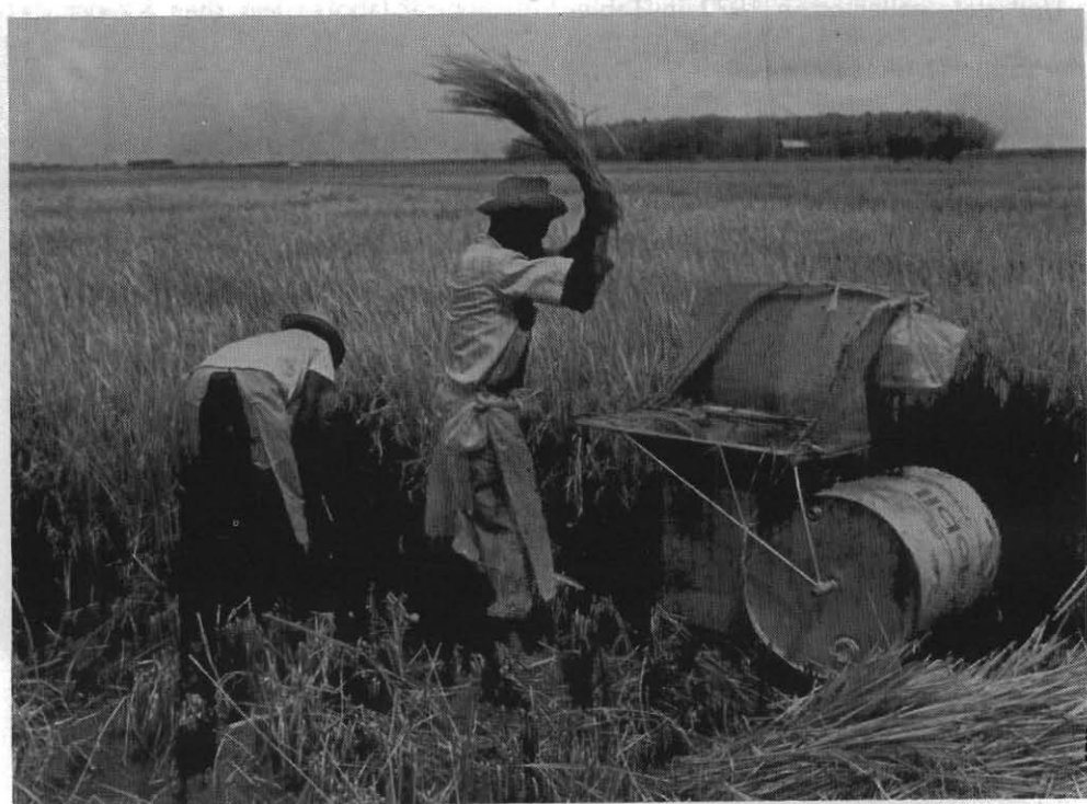
A portable, man-powered rice combine, designed at CIAT, increases labor efficiency.
