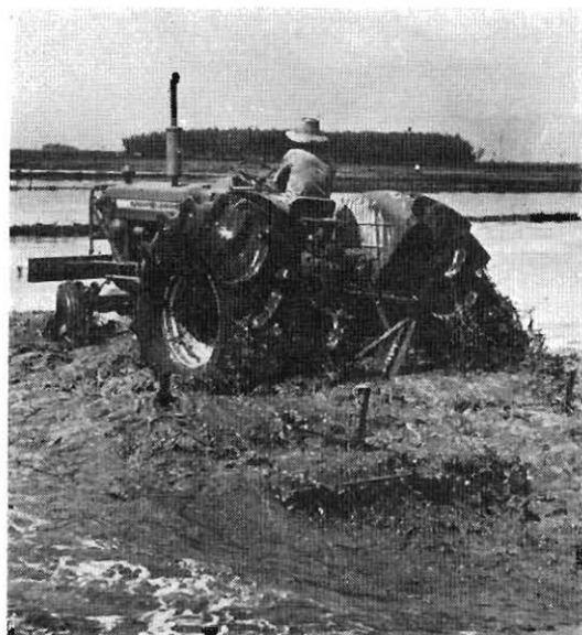
Land levelling under water with a spike tooth harrow.
