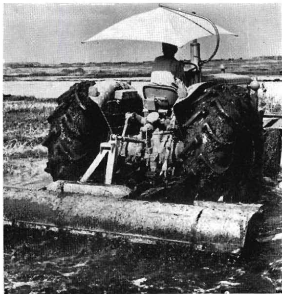
Preparing wet land with a prototype rotary tiller.
