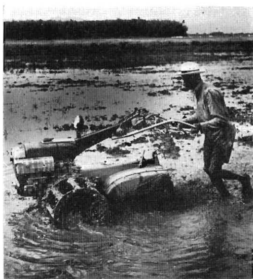
Land preparation under water with a small 8 h.p. tractor.
