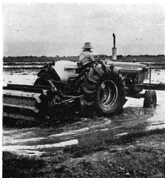
Testing of a powered cylinder for land preparation under water.
