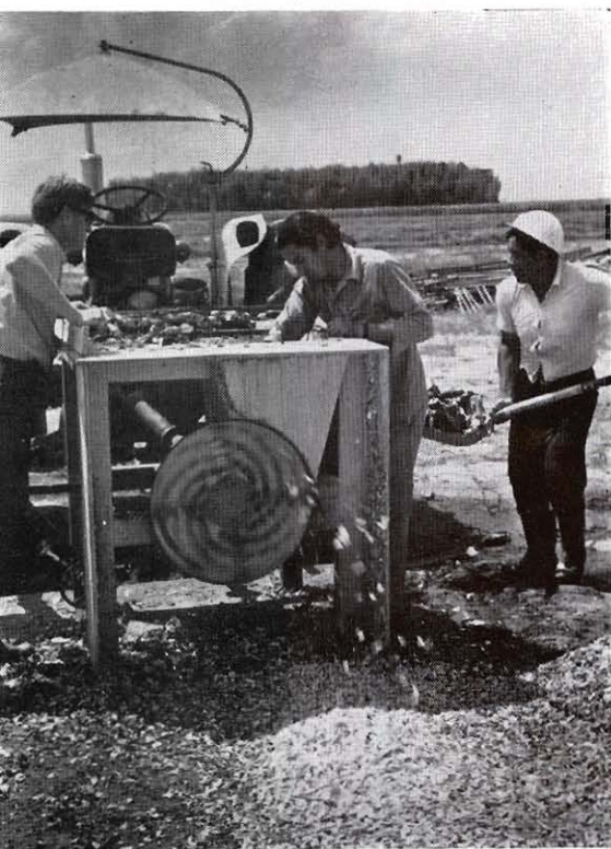
FIG. 1. Testing the "barrel head" cassava chipper, which uses a tractor for power.
