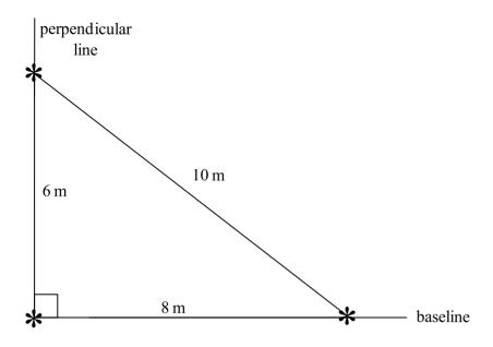
Figure 2. A simple way of setting out a 90-degree corner in field experiments.
