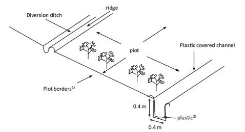
Figure 8. Experimental layout of simple trials to determine the effect of soil/crop management practices on
