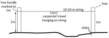
Move one hoe until bubble in carpenter's level is in the center.
