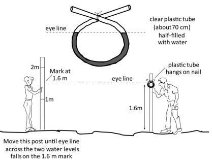
Figure 12. Simple method to set out contour lines using a plastic tube with water: the "buffalo horn".
