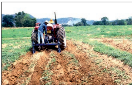
To improve drainage, a "subsoiler" can be used to break the compacted subsoil.
