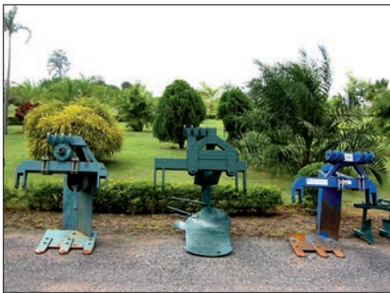
Several types of tractor-mounted cassava harvesting tools are available in Thailand.
