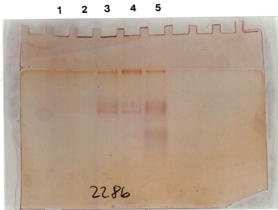
Figure 5a. Staining for acid phosphatase (ACP). (15% homogenous gel, 0.5 M Tris/HCl (pH 8.8) as tank puffer, 100 V, 210 minutes running time).
