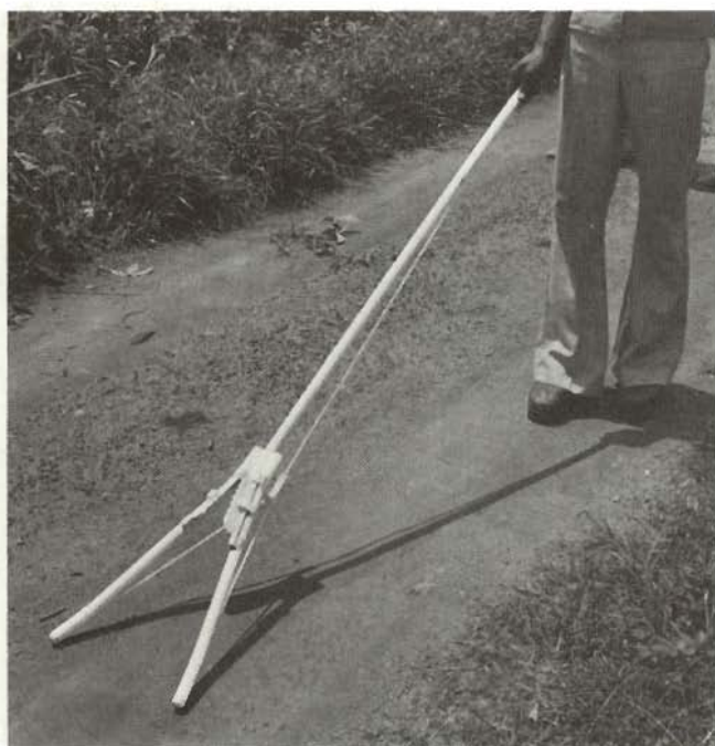
A simple lever designed at IITA to make harvesting easier. (Source: R. Wijiwardene)
