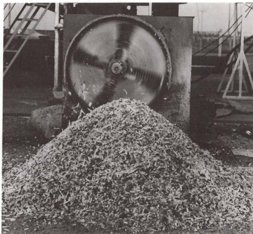
Malaysian-designed chippers produce cassava chips with the optimal shape for fast drying. (Source: CIAT)
