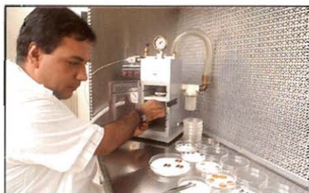
Figure 6. CIAT staff are using biolistics to transform Brachiaria , common bean, and rice. One such approach involves the use of a PDS-He/100 helium-driven particle accelerator, which bombards regenerative tissues with DNA-coated microprojectiles.
