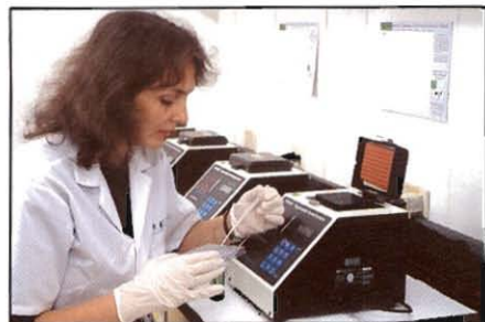
Figure 1. A thermocycler makes millions of copies of DNA from a small sample by means of PCR.
