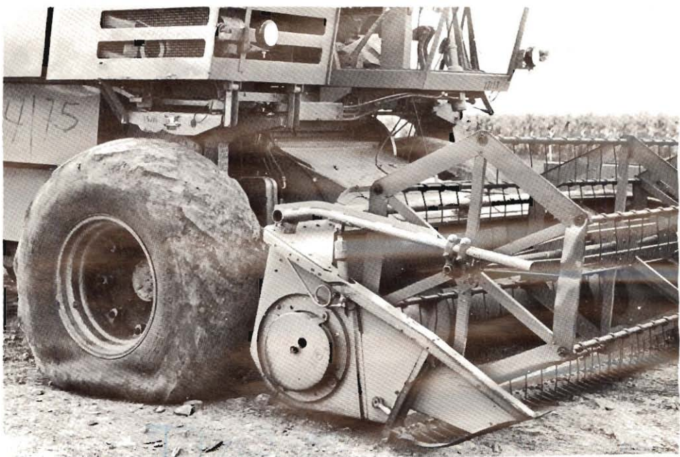
Figure 5. A smooth tire inflated to a low pressure provides improved mobility for this combine in soft soils at CIAT.
