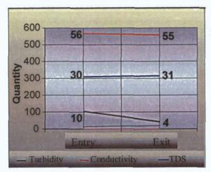
Figure 18. Effects of the wetland on the quality of water (TDS = total dissolved solids).
