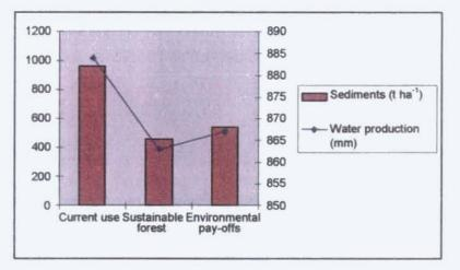
Figure 11 Simulated annual averages of sediment and water production in three scenarios, Jalapa watershed, Honduras.
