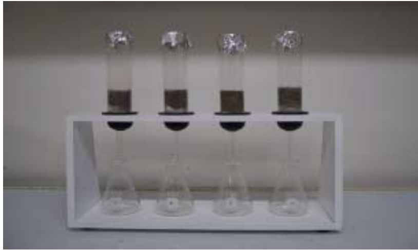
Photo 2. Leaching Tube Setup
