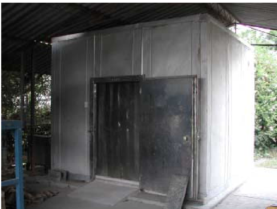
Figure 1.3. Photograph of the chamber with controlled temperature and relative humidity for more reliable and comparable measurements of PPD.
