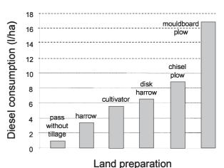
Figure 10.2. Diesel fuel consumption while performing different tractor operations (after Nalewaja 2001).
