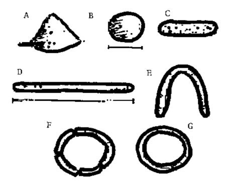
Fig. 6.4 Point at which the soil becomes malleable and can be hand-shaped, indicates its texture. (Source: Agricultural Compendium for Rural Development in the Tropics and Subtropics)
