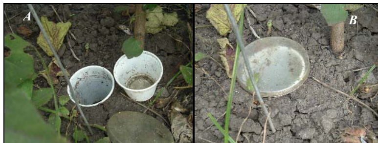
Figure 1. (A) Fixed component and removable component and (B) lid of the pitfall traps in the field.
