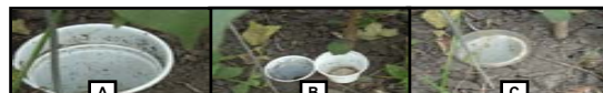
Fig. 1. Pitfall traps showing (A) fixed component, (B) removable component and (C) lid.
