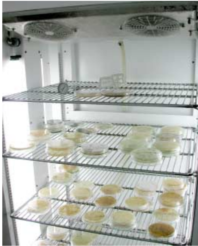
Figure 7.1. Incubator for culturing and multiplying isolates of fungal entomopathogens.
