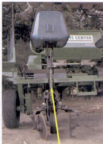
*Photo 5. Spring device to control planting depth of the cassava stake.*
