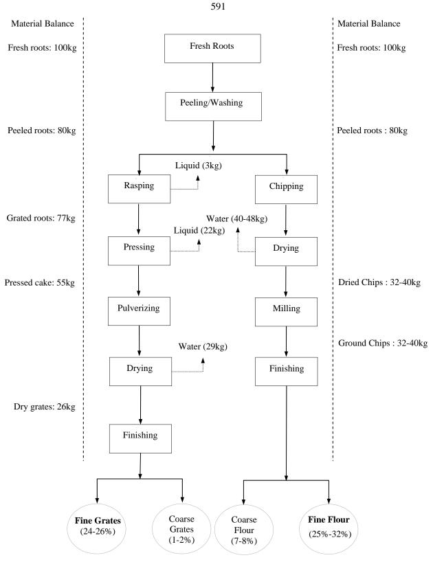
Figure 1. Cassava flour and grates processing flow and estimated recovery (in percent) from fresh roots.
