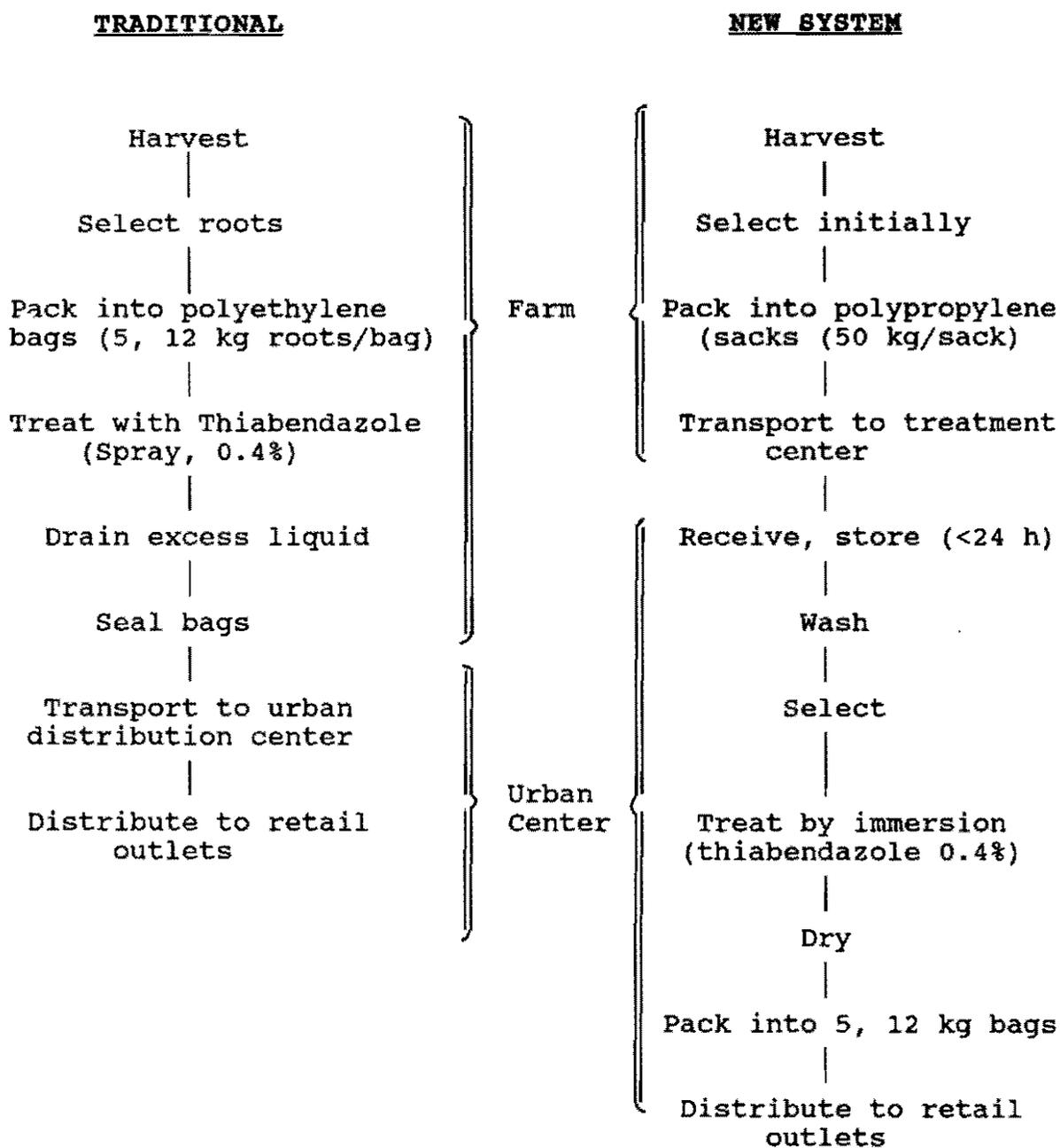
Figure 7.2 Traditional and new processes for fresh cassava root storage.
