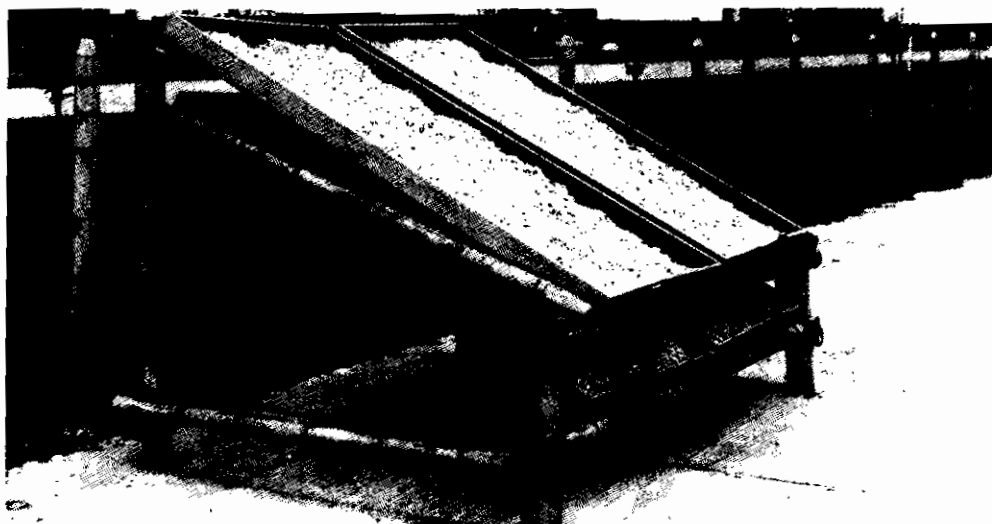
Figure 68. When inclined trays are stacked in this way with a 30-centimeter space between them, drying rates for the chips are not appreciably affected.
