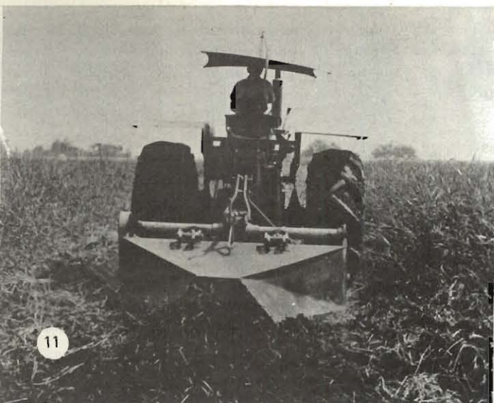
The levee maker mounted on the rear of a rototiller in action.
