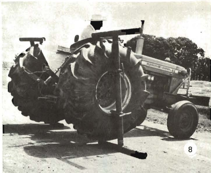
Four-inch pipe attachment in form of "I" designed and built in CIAT to increase traction when bogged. When used always operate tractor in reverse to prevent accidents.
