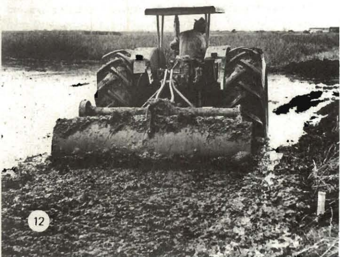
Leveling high spots with a blade mounted on the rear of a rototiller.
