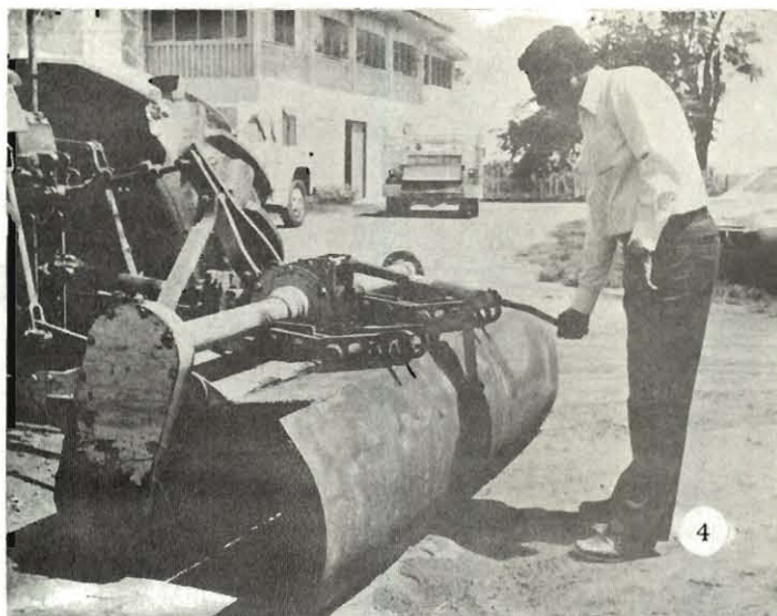
Blade mounted on rear of rototiller for cutting and movement of soil.
