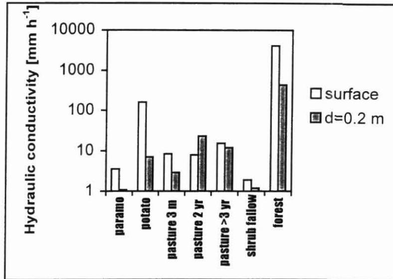
Figure 12. Saturated hydraulic conductivity of soils under different land uses at depths of 0 and 0.2 m, as estimated in the field using infiltration experiments.
