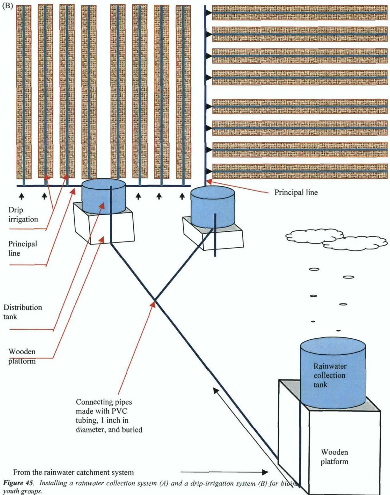
**Figure 45.** Installing a rainwater collection system (A) and a drip-irrigation system (B) for bioinspired youth groups.
