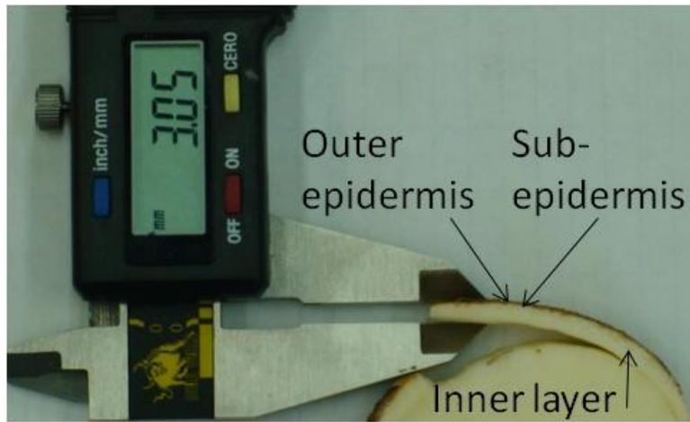
**Figure 1.** Illustration of a section of the cassava roots showing the three components of the phelloderm or “peel” and the digital caliper used to measure it.
