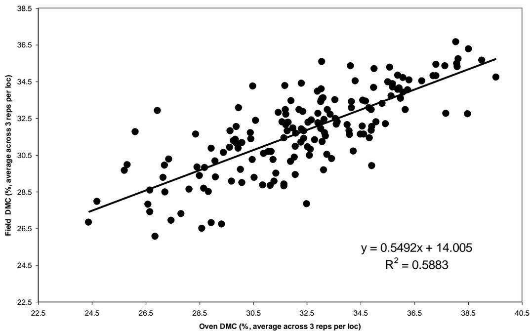
**Figure 3.** Relationship between DMC estimated by the oven and by the gravimetric methods. Divergence of results tended to be larger at low levels of DMC (< 33%). Each data point represents the averages (across three replications) for each clone at each location (total of 33 clones x 5 locations = 165 data points)
