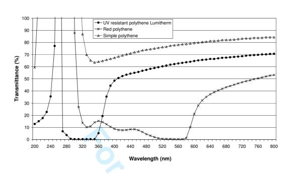
Figure 1. UV/visible spectrum of polythene sheeting used in drying studies.
