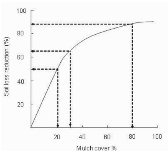
Figure 10.3. The relationship between mulch cover and loss to soil erosion.
