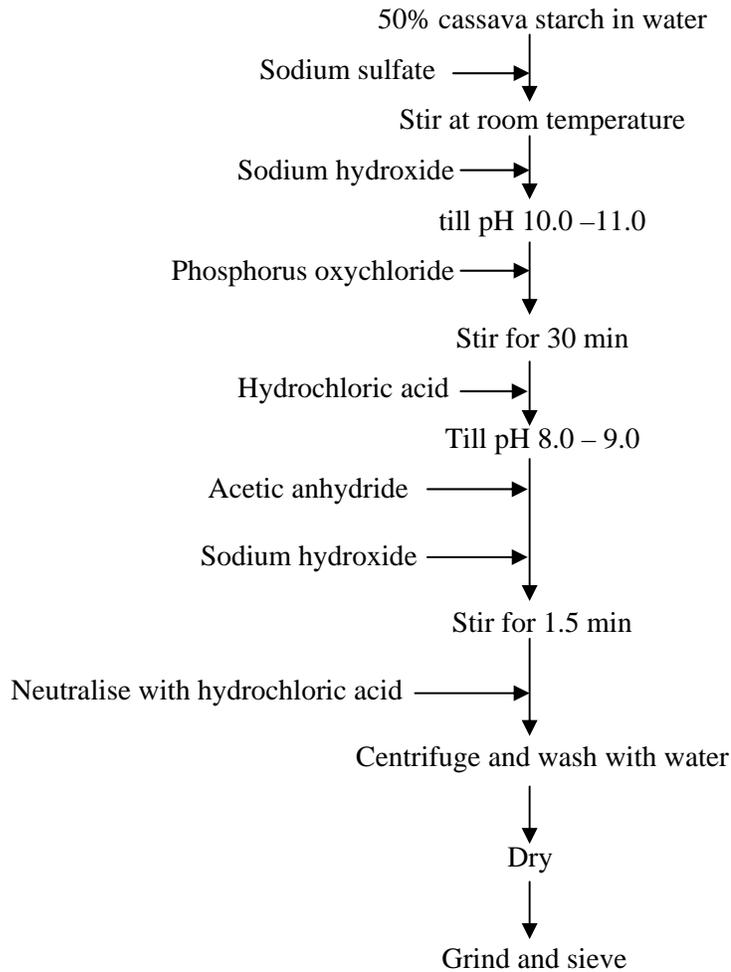
Figure 3: Preparation of cross-linked acetylated cassava starch.
