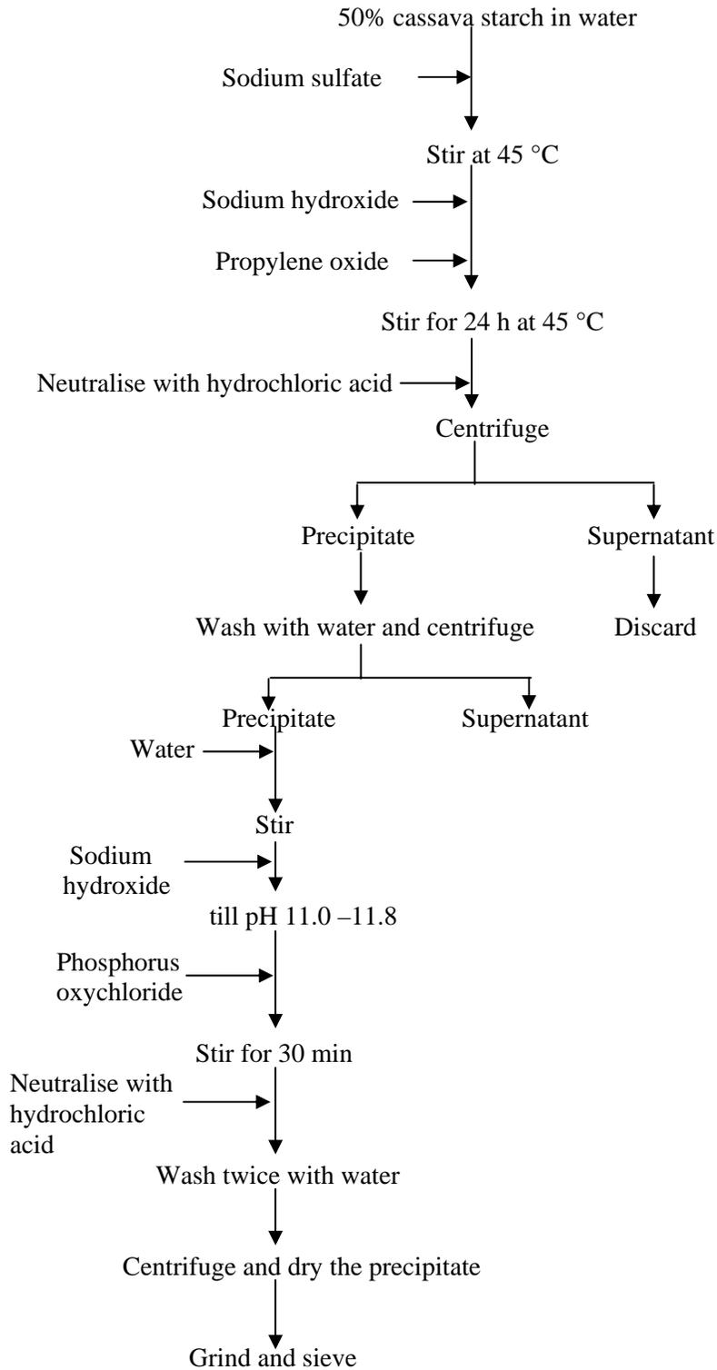
Figure 2: Preparation of cross-linked hydroxypropyl cassava starch.
