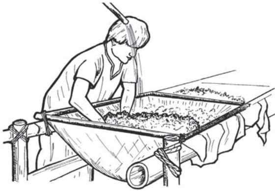
Figure 26-12. Manual sieving of the grated cassava mass, as performed in the department of Cauca.
