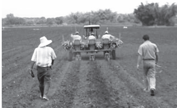
Figure 20-9. Three-furrow cassava planter, model PMT-3.
