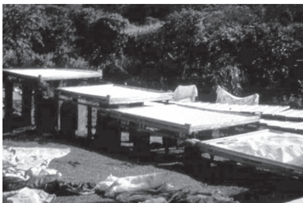
Figure 26-17. Sour cassava starch drying system in some of the extraction plants in the department of Cauca.
