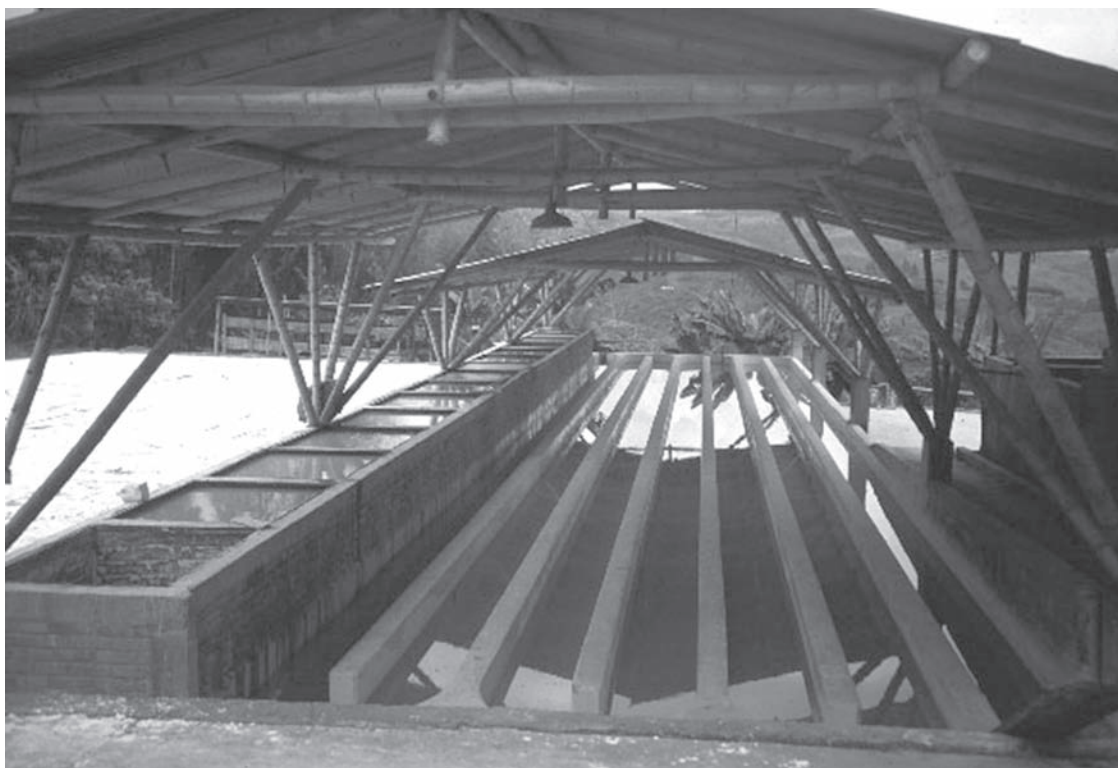
Figure 26-15. System of 7 channels for starch sedimentation of starch milk.
