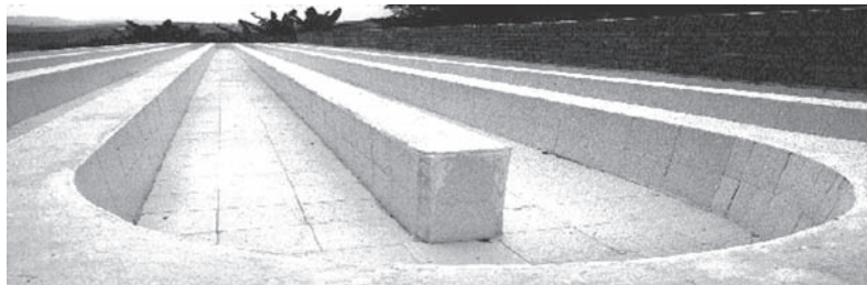
Photo 26A-11. Starch sedimentation channels.
