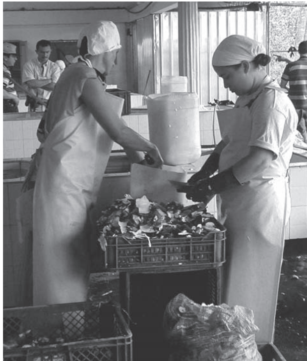
Figure 25-24. Removal of tips and chopping roots into cylinders.
