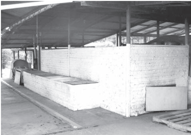
Figure 22-14. CLAYUCA's artificial fixed-bed dryer at CIAT, Palmira.
