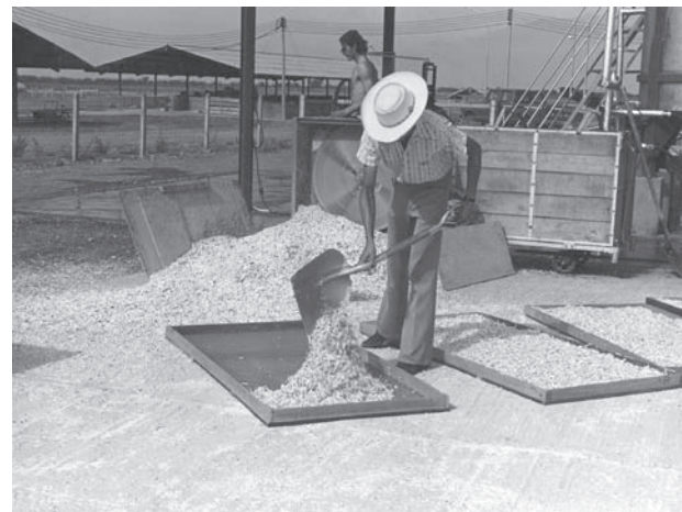
Figure 21-27. A worker fills the trays with fresh cassava chips as a chipping machine operates behind him.
