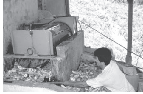
Photo 26A-8. Semi-continuous mechanical root washing.
