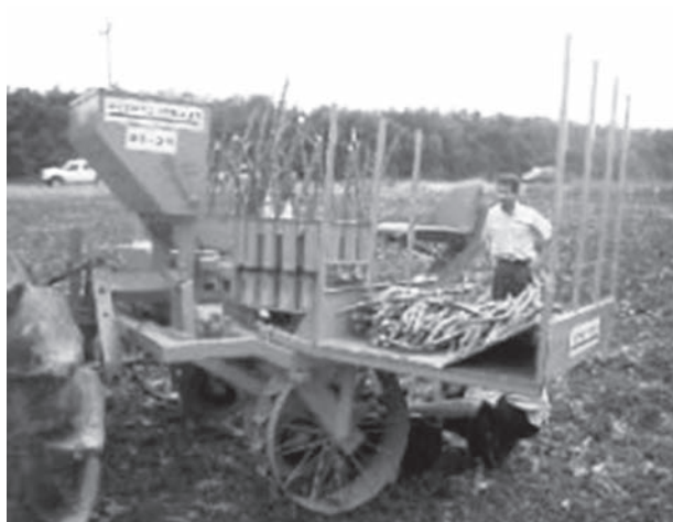
Figure 20-8. Two-furrow cassava planter, model PC-20.
