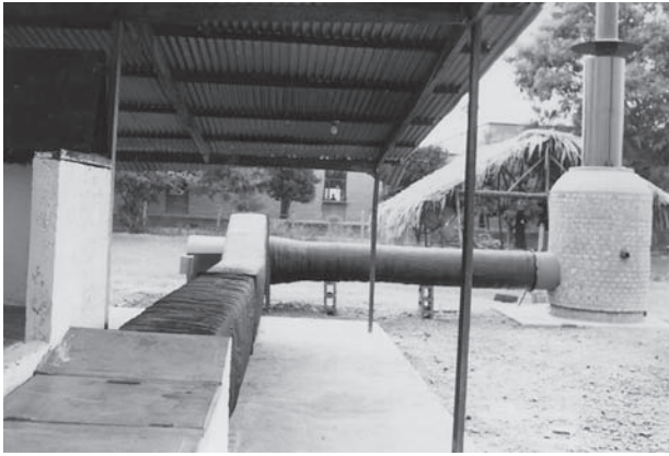
Figure 22-3. An artificial fixed-bed dryer that uses a coal burner to heat the air.
