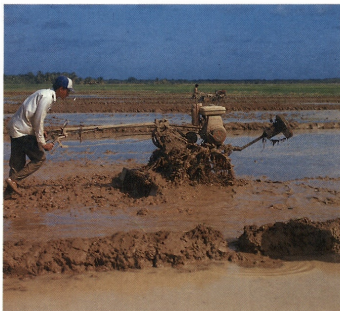
This small, motorized cultivator, designed by IRRI, has been tested in the Dominican Republic. Here, it is being used for soil leveling.
