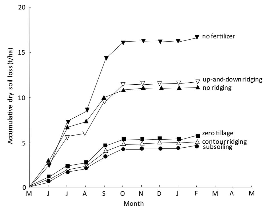
**Figure 6. Effect of various soil/crop management practices on the accumulative dry soil loss by erosion on 7% slope at Sri Racha Experiment Station, Thailand, during a 9-month growth cycle of cassava in 1988/89.**
