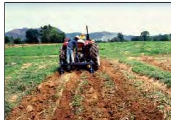
Photo 7. Using a subsoiler to loosen the compacted subsoil in Thailand
