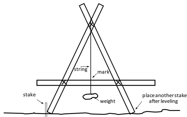
Figure 10. A-frame to set out contour lines.
