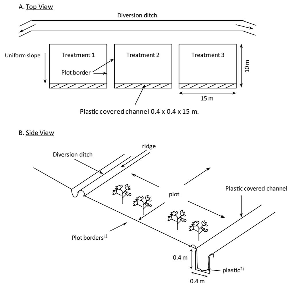
Figure 8. Experimental layout of simple trials to determine the effect of soil/crop management practices on soil erosion.
