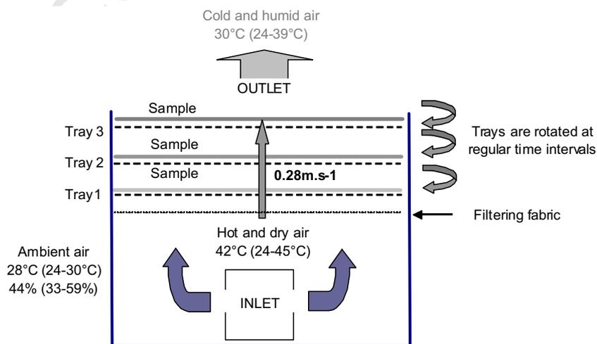
Fig. 1. SSec-T® cross flow dryer (temperature/humidity: mean (min–max)).
