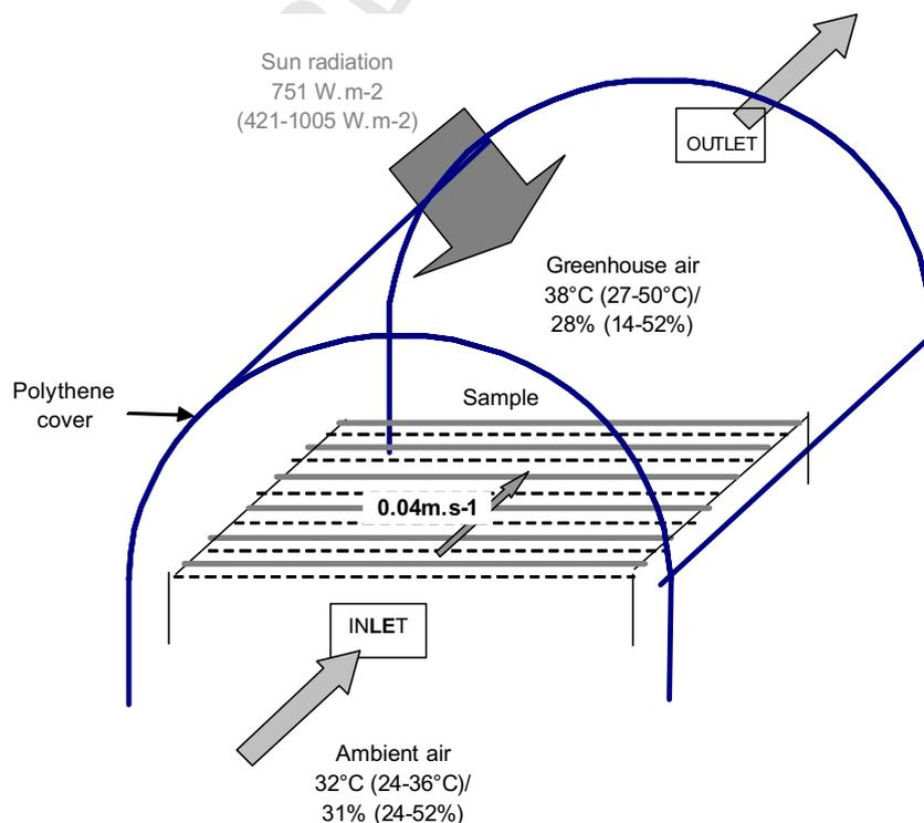
Fig. 2. SCec-Serre® greenhouse solar dryer (temperature/humidity: mean (min-max)).
