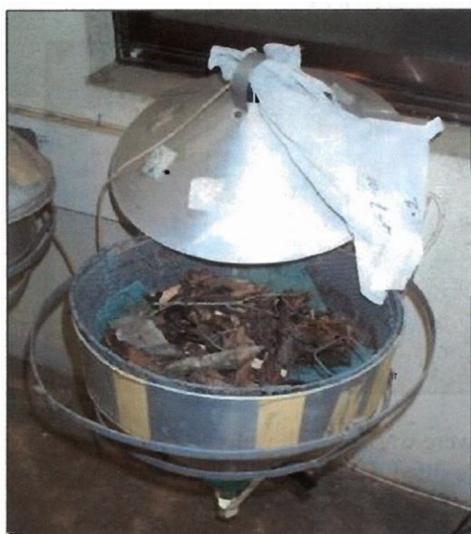
Figure 2. Berlese funnel filled with soil and litters.
