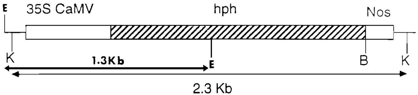
Figure 1. Gene constructs used in co-transformation of rice.
