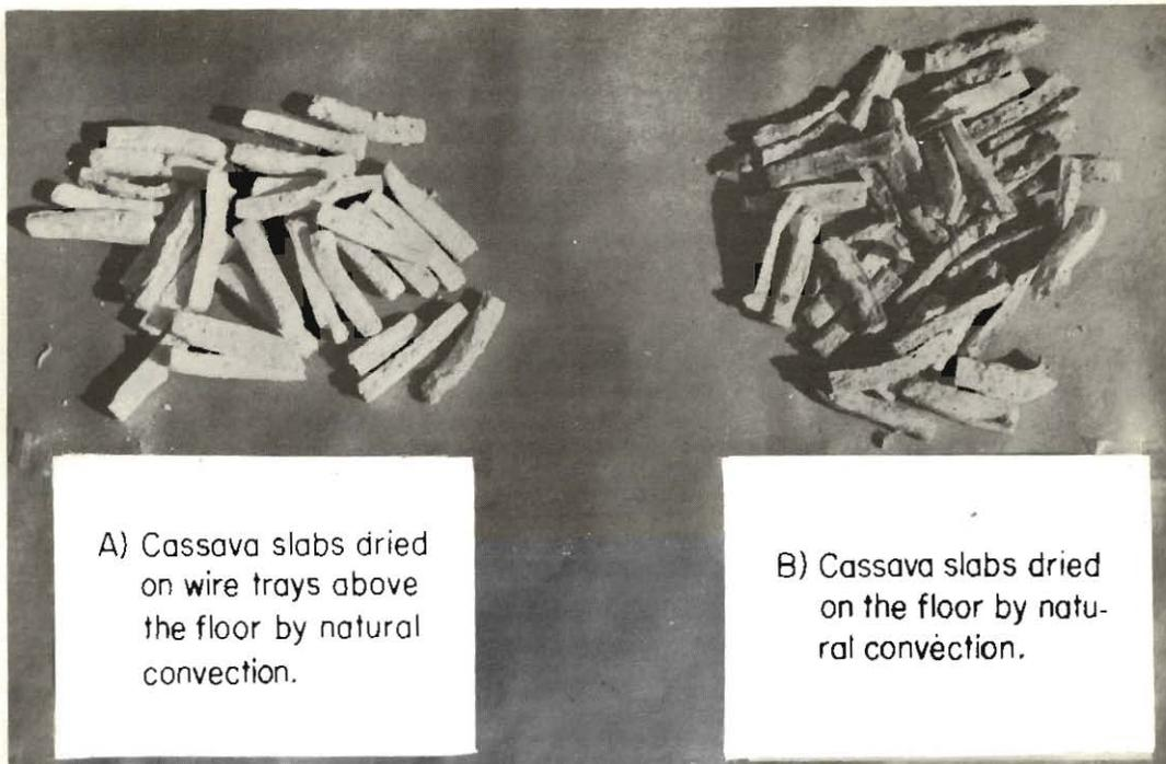
A) Cassava slabs dried on wire trays above the floor by natural convection.
