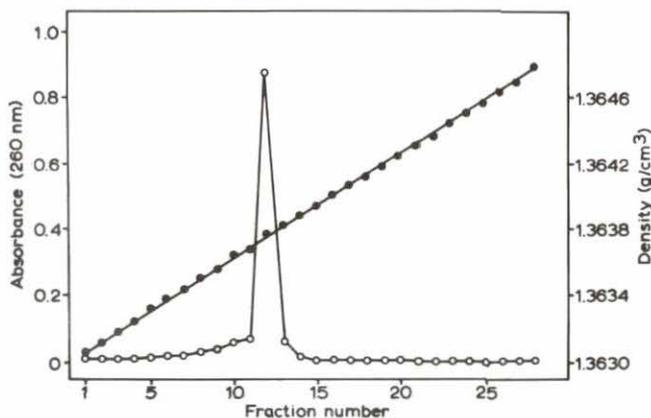
Fig. 17. UV-absorption pattern of the fractions collected after equilibrium centrifugation of BMMV-CIAT in caesium sulphate. • = density of the fractions; o = absorbance at 260 nm.
