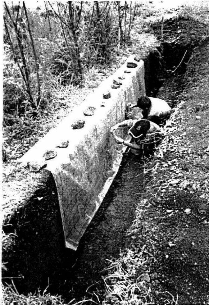
Figure 9. Root mapping: details about preparation of pits and location of PVC sheets on pit wall.
