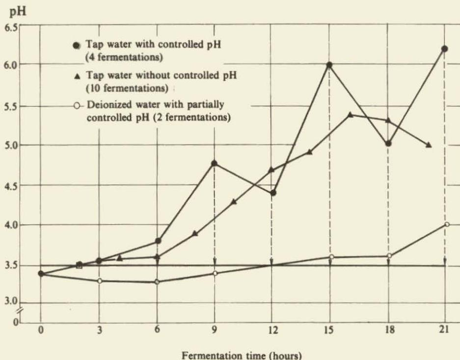
Figure 4. Change in pH during the fermentation of wole cassava media (in tap and deionized water) by *Aspergillus fumigatus* I-21A, with and without the addition of 9N sulfuric acid
