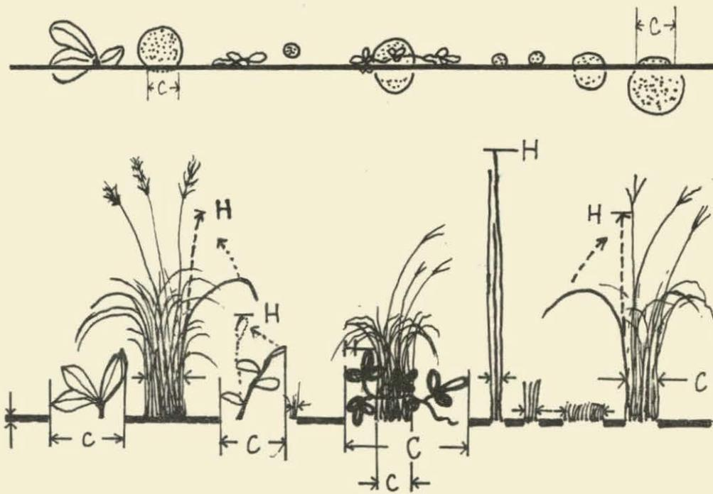
Figure 1. Measuring method of plant height and coverage
